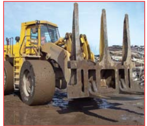
The company's new 115ZV-2 replaced a Komatsu. It is used primarily to unload and move scrap car bodies.
