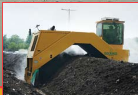
A Backhus turns the windrows. In 60-75 days the compost is ready for screening.
